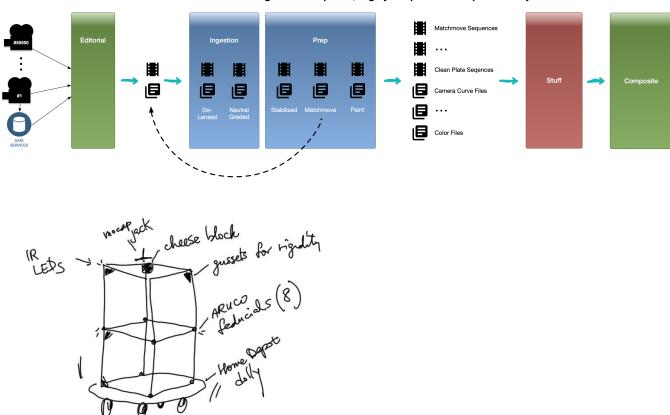
Calibration gadget. vertices are spaced at exactly 1m joined by aluminum extrusion
