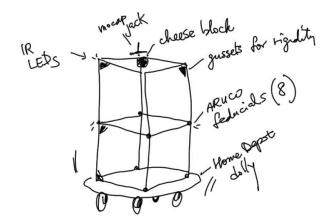
Calibration gadget. vertices are spaced at exactly 1m joined by aluminum extrusion
